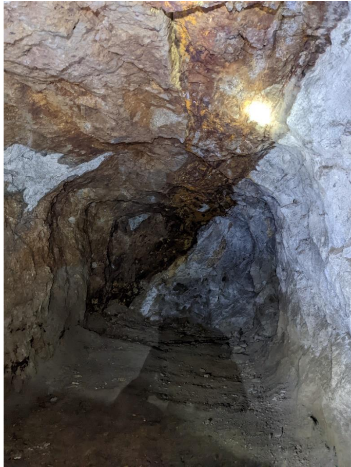
Underground in the mine – sharp ore waste contact
